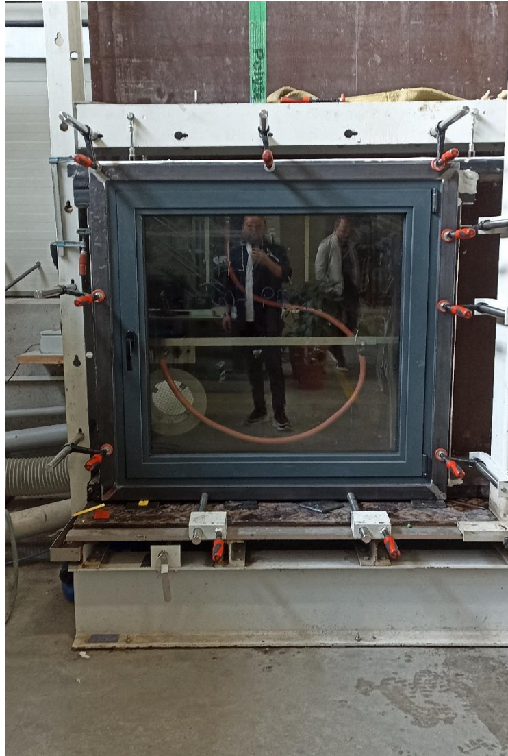
Resim No. 1 Monte Deney Numunesi / Fig. No.1 Mounted Test Specimen
